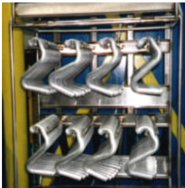
Tubes Racked for cleaning
